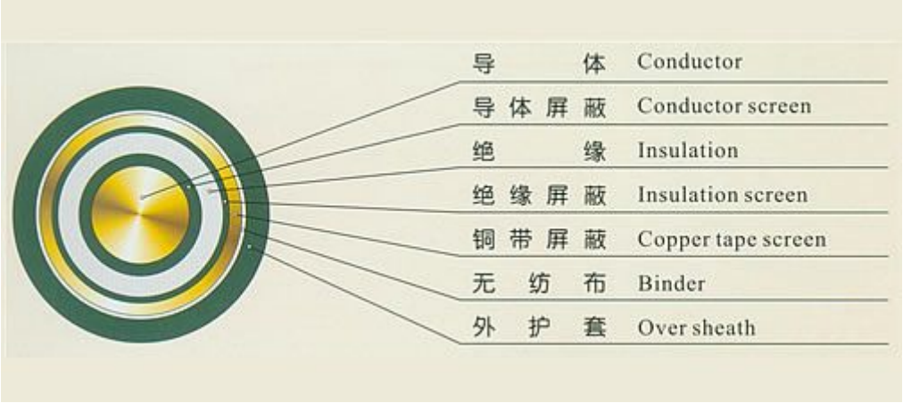
Single core XLPE insulation power cable for rated voltage from 3.6/6kV to 26/35kV
